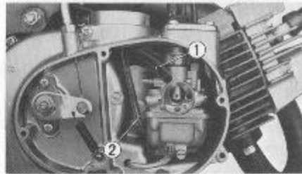
① Fuel hose ② Air vent hoses
